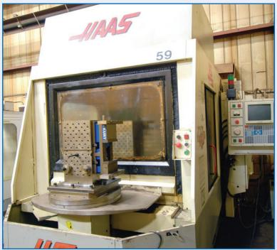
HAAS HS-1 CNC HORIZONTAL MACHINING CENTER
