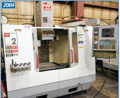
HAAS VF2D CNC VERTICAL MACHINING CENTER
